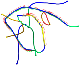
Fig. 8. Tensor field design based on purely user-specified constraints (curves with spikes) can lead to excess degenerate curves (without spikes).
